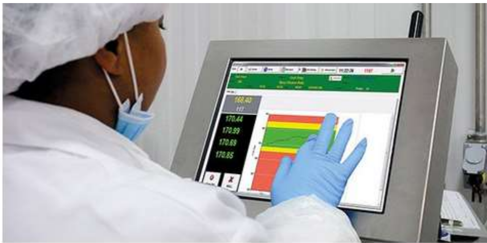
Figure 1 Cooked Product Continuous Temperature controlling system
